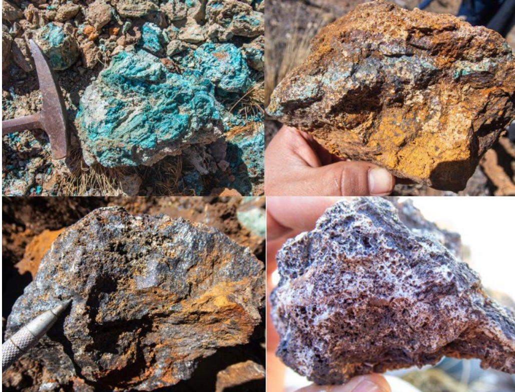
Figure 4 – (Top Left) Garnet skarn with copper oxides, Rock sample P017010 assayed 2.82% copper; (Top Right) Garnet-magnetite skarn with copper sulphides and oxides, Rock sample P017020 assayed 1.11% copper and 0.19g/t gold; (Bottom Left) magnetite skarn, Rock sample P017021 assayed 1.13% copper and 0.17g/t gold; (Bottom Right) Quartz boxwork vein with goethite and hematite, a cutting marbleized limestone of the Ferrobamba Formation, rock sample P017045 assayed 2.55g/t gold, 19.3ppm molybdenum and 264ppm arsenic.
