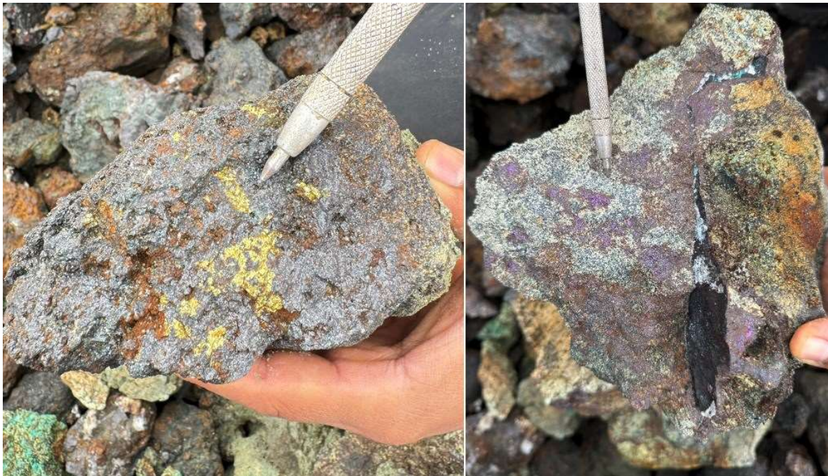
Figure 5 – (Left) Magnetite skarn with strong chalcopyrite mineralization. (Right) Magnetite skarn with strong bornite mineralization.
