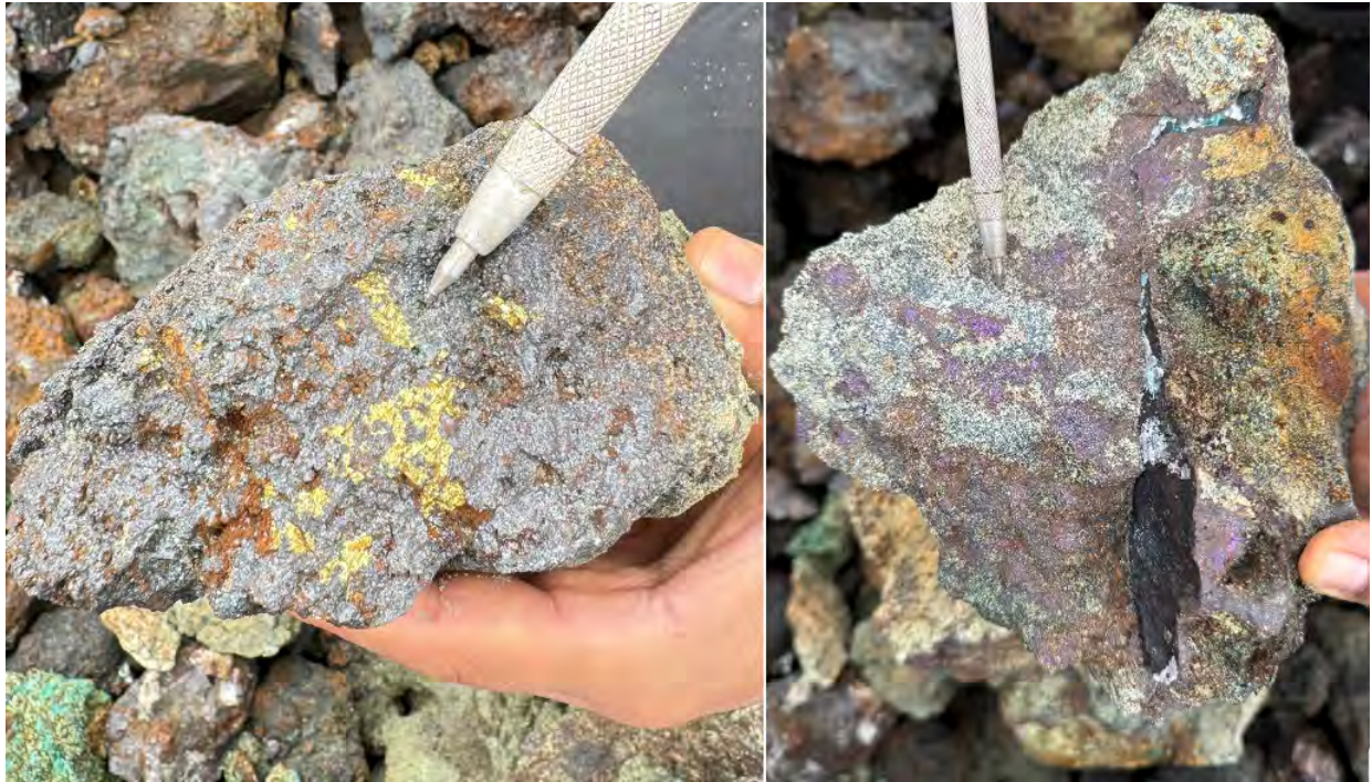
Figure 2: (Left) Magnetite skarn with strong chalcopyrite mineralization. (Right) Magnetite skarn with strong bornite mineralization.
