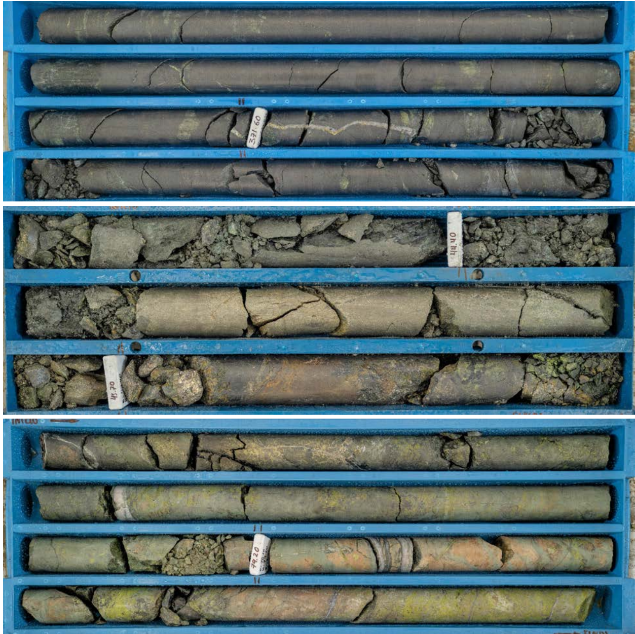
Figure 1: (Top) KHZ5825-003 Massive magnetite skarn cut by quartz-chalcopyrite-bornite veinlets and with disseminated chalcopyrite. The 1.7m interval assayed 0.67% copper, 0.063 g/t gold, 1.82 g/t silver and 122 ppm molybdenum from 370.9m to 372.6m downhole depth. (Middle) KHZ5790-001 Garnet-diopside skarn cut by pyrite-chalcopyrite mineralization. The 1.9m interval assayed 1.38% copper, 0.27 g/t gold, 7.14 g/t silver and 5 ppm molybdenum from 43.9m to 45.8m downhole depth. (Bottom) KHZ5790-001 garnet-diopside skarn with strong chalcopyrite mineralization, and cross-cutting quartz sulfides veinlets. The 1.4m interval assayed 4.91% copper, 0.42 g/t gold, 17.35 g/t silver and 164 ppm molybdenum from 77.1m to 73.5m downhole depth.
