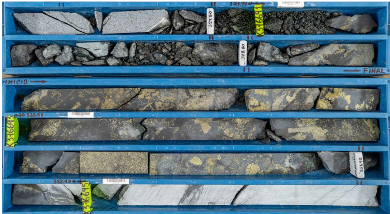
Figure 3. Drill core from KHZ5140-001, showing high-grade, manto-style copper mineralization that assayed 2.97% copper over 4.2 metres.
