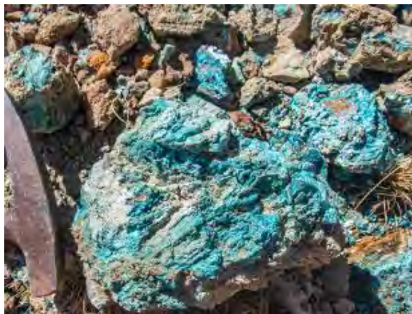
Garnet skarn with copper oxides, assayed 2.82% copper
