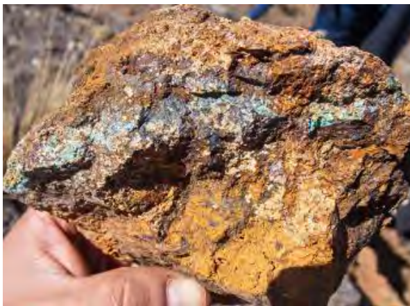
Garnet-magnetite skarn with copper sulphides and oxides, assayed 1.11% copper and 0.19g/t gold
