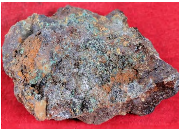
Skarn with bornite assayed 2.61% Cu, 0.11g/t Au
