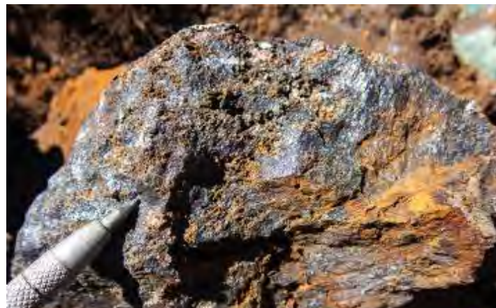
Magnetite skarn, assayed 1.13% copper and 0.17g/t gold
