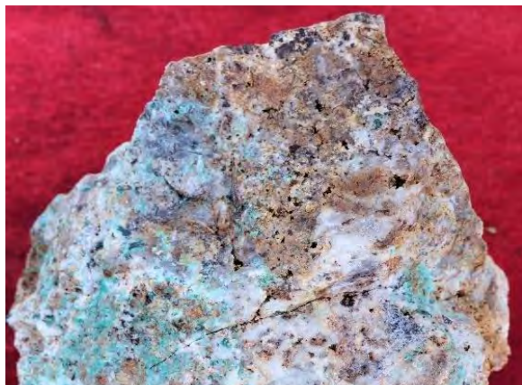
Epithermal quartz breccia assayed 2.60% Cu, 6.0g/t Au
