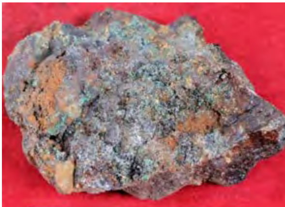
Skarn with bornite assayed 2.61% Cu, 0.11g/t Au
