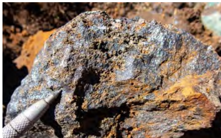
Magnetite skarn, assayed 1.13% copper and 0.17g/t gold
