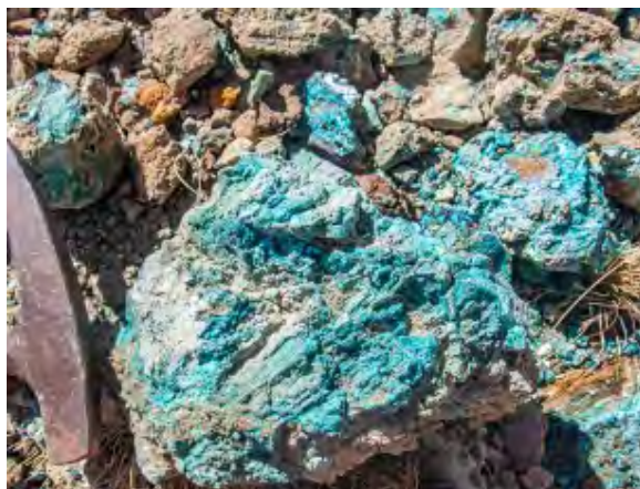
Garnet skarn with copper oxides, assayed 2.82% copper
