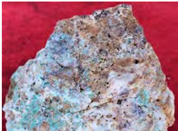
Epithermal quartz breccia assayed 2.60% Cu, 6.0g/t Au
